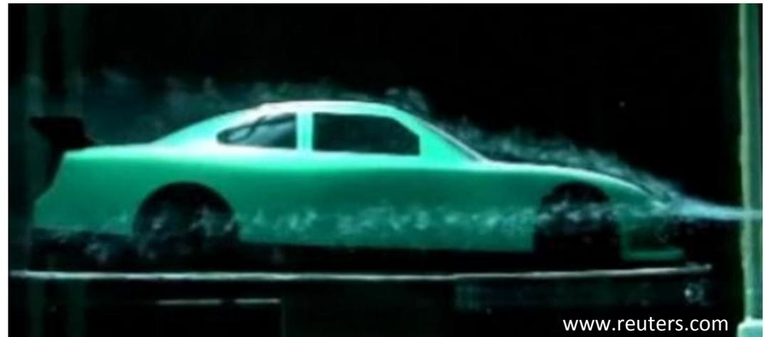
Race car being tested in a water tunnel
