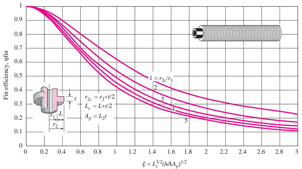
**FIGURE 10-43** Efficiency of annular fins of constant thickness  $t$ .
