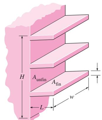
$$\begin{aligned} A_{\text{no fin}} &= w \times H \\ A_{\text{unfin}} &= w \times H - 3 \times (t \times w) \\ A_{\text{fin}} &= 2 \times L \times w + t \times w \\ &\approx 2 \times L \times w \text{ (one fin)} \end{aligned}$$
