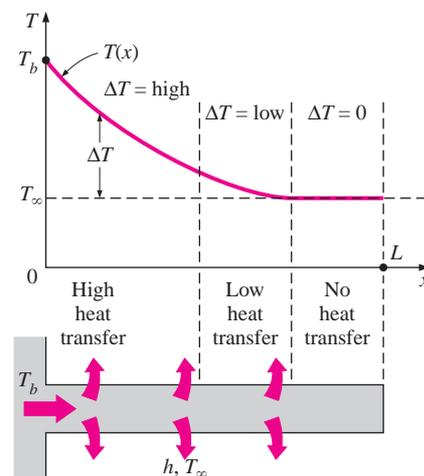
**FIGURE 10-46** Because of the gradual temperature drop along the fin, the region near the fin tip makes little or no contribution to heat transfer.
