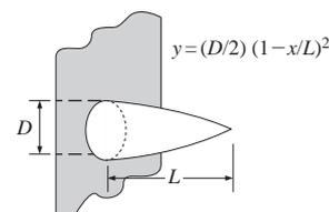
**Pin fins of parabolic profile
