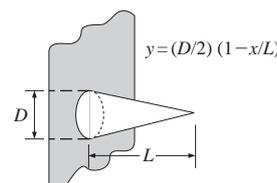
**Pin fins of parabolic profile**
