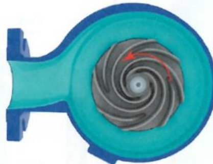
(c) Radial, open-type impeller in the rear part of its pump case. Fluid enters at the center of the impeller (called the eye), is thrown radially outward by the vanes, travels around the volute, and exits through the discharge port at the left. Rotation is counterclockwise. The front part of the case contains the suction port and completes the volute.
